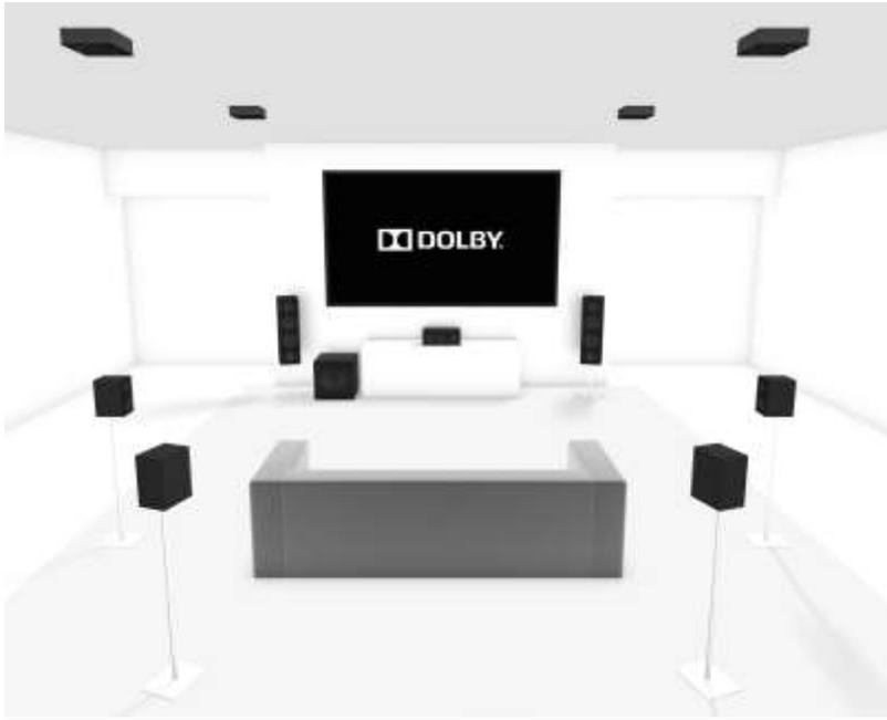
Figure 5: If you use ceiling speakers, Dolby recommends using four or more.
